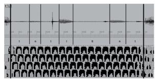
Figure 2: Acoustic waveform and EPG linguopalatal profiles during the homorganic word [tntlttnt] "you hid them (fem.)". The four lines show the electrodes contacted (i.e. black squares).
