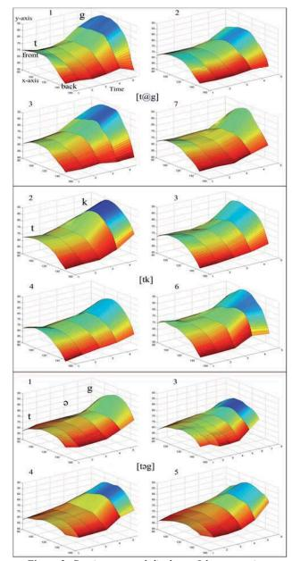
Figure 3: Spatio-temporal displays of the successive tongue shapes over time (derived from kriged contours) for 4 representative tokens of [t@g], [tk], and [təg].
