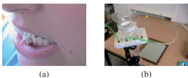
Figure 2: (a) Attachment of tube to lower incisor, and (b) to hand-held transducer interface.
