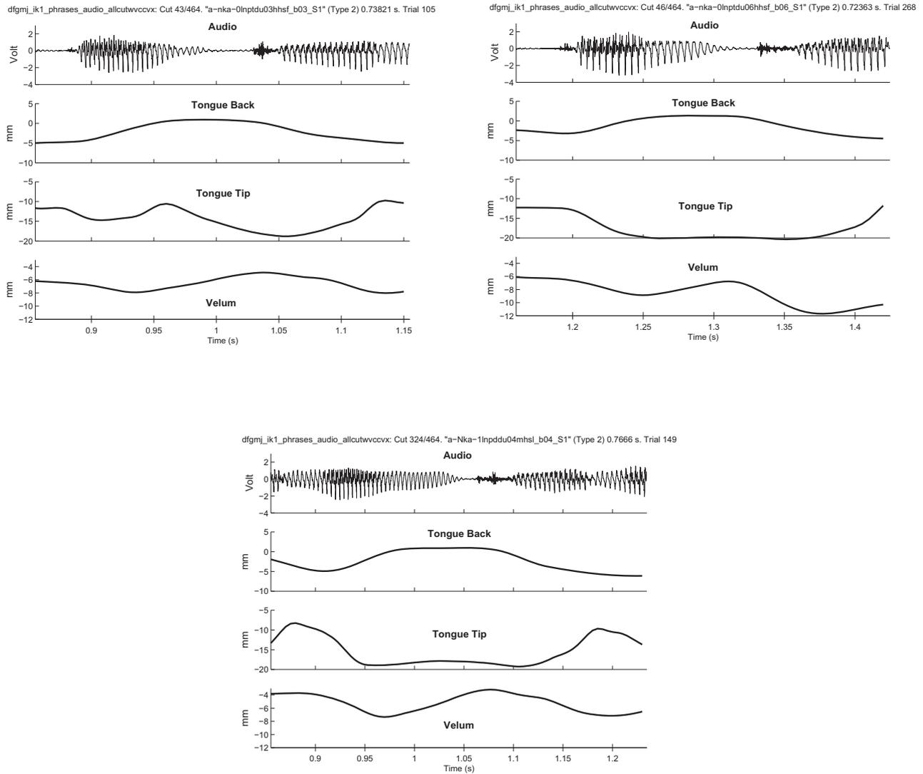
Figure 2: Illustration of "dann kann" with visible tongue tip excursion (left chart, top) and without visible tongue tip excursion (right chart top) during the nasal-plosive closure phase and control "lang kann" item (bottom).
