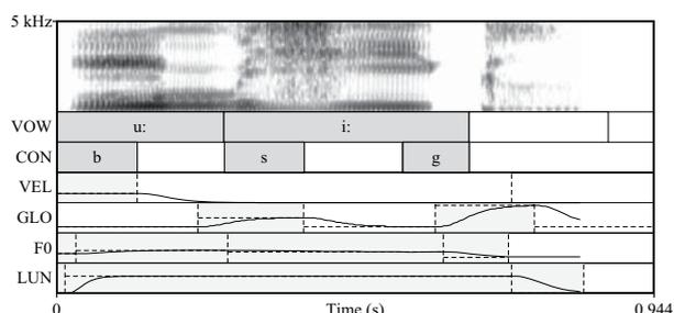
Figure 1: *Synthesis result and gestural score for the utterance Musik [mu:'zik]. The [m] is produced with bilabial occlusion (the **b** gesture) and lowered VELum. The **s** and **g** gestures, combined with the GLOttal gestures, produce [z] and [k], respectively.*
