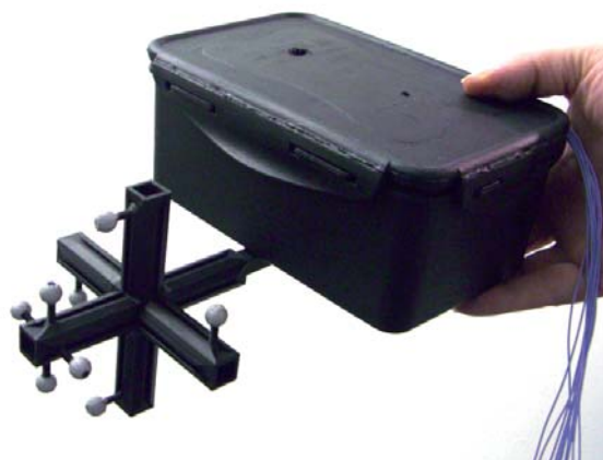
Figure 2: The SMC with the OPT markers at the end of the 3D cross structure extension
