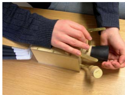
Figure 1: Photograph of the inner life of the speaking machine while being played: palm of the hand on the right forming vowel resonances in front of a rubber funnel (vocal tract); the hand on the wooden windchest (thorax) regulating nasal cavity resonances; (invisible) elbow providing pressure on the bellows (lungs). The reed pipe is located within the "nose".
